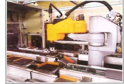
Vision Inspection on silicon wafers
