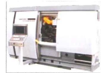
Integrated Robot inside machine tool
