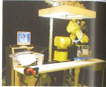
Robot picks up a sheet metal on moving outfeed conveyor from press machine. Using multiple camera information, robot detects large size work location and orientation on conveyor.
