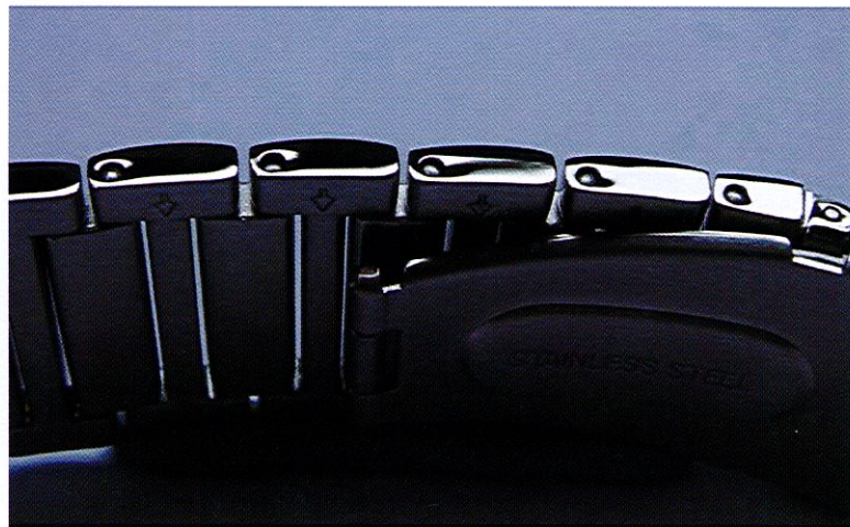
Figure 6.3 Edge effects around holes (Courtesy of Mr. John Mak)
