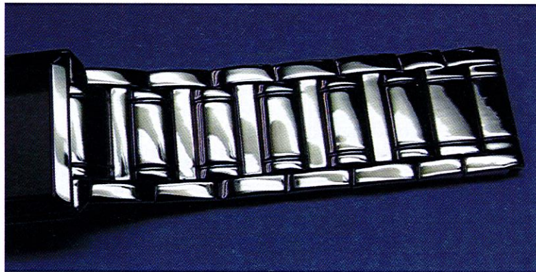
Figure 6.1 Surface waviness after buffing (Courtesy of Mr. John Mak)
