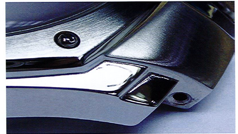
Figure 6.4 Inaccessible concave corners (Courtesy of Mr. John Mak)
