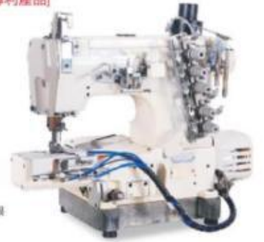
BAF 自動折袖口縫紉裝置, 對射電眼 Automatic folding cuff device, Correlation sensor
