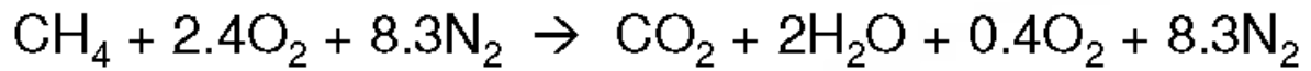
Equation 1: Chemical combustion reaction of methane (one of the components in Town gas)
